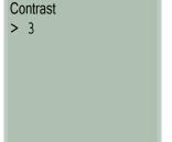
The display contrast is pre-caliblrated, however can be adjusted here if desired. This setting makes the entire display lighter or darker.
